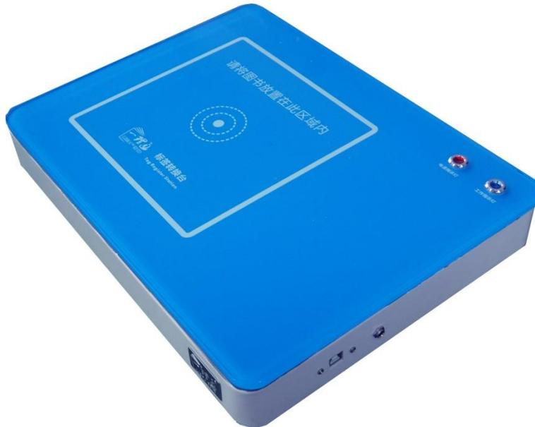
Tagging Workstation also known as the conversion station which converts the accession number / barcode placed on items to an RFID tag which will be the medium of item identification for circulation using an RFID enabled station.
